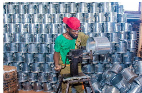
Kavuuma Paul at work. The insulated charcoal stove is made of galvanized metal sheet, clay liners and insulating materials. Photo: TARD
