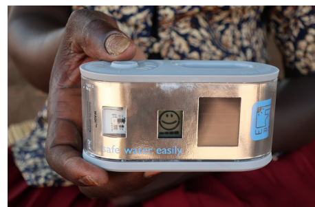
WADI functions as an UV indicator showing the users a smiley face when the solar disinfection process is completed. Photo: Barbara Oberfichtner/Helioz
