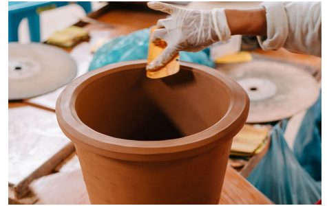
The purifiers are mixed from local clay and rice husks and pressed into a mould. Photo: TerraClear
