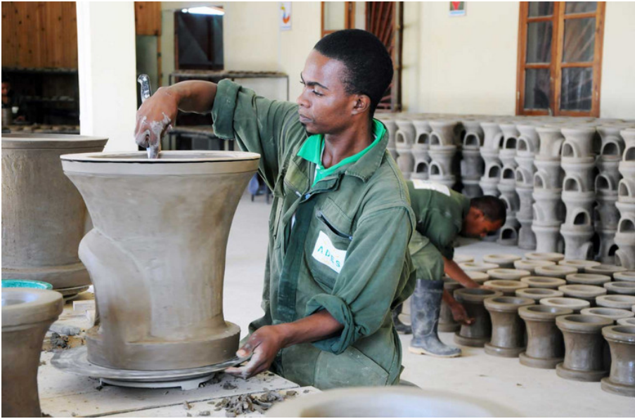
Benjamin Rakotovaomanana on completion of a clay combustion chamber for schools. Photo: Angela Zimmermann
