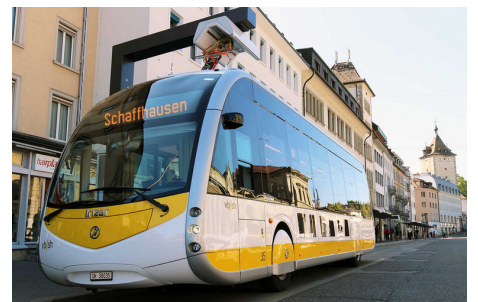
The VBSH e-bus with rapid charging system draws energy from a battery installed on the roof, which is charged in a very short time both in the depot and at individual stops. Photo: Christoph Wahrenberger
