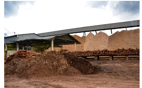
Stockpiled sawdust (in the back) and wood logs ready to be chipped and mixed with the biomass residues in order to be fed into the biomass boiler.
