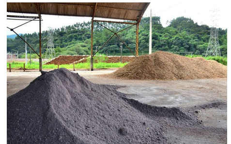
Stockpiled biomass residues from forestry activities (background) and sludge from the mill's processes ready to be mixed and then sent to the biomass boiler.
