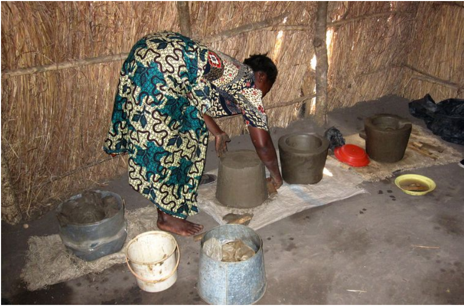
Rural women groups manufacture the portable ceramic stoves at village level. Here a women brings clay into shape to form the stove in Thawale village in Southern Malawi.
