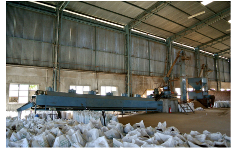
Pellet factory: Biomasse is processed into pellets for the efficient stove.
